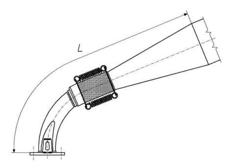
To achieve this dimension, the flexible (supplied with the engine) must be cut at a length of **50÷60mm** (flexible completely closed).
