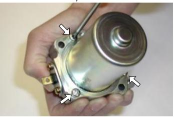
REMOVE DRUM FROM STARTER **KEEPING ROTOR IN ITS SEAT** (BE SURE TO HOLD THE ROTOR ON ITS TOOTHED SIDE TO PREVENT BRUSHES THE BRUSHES MAY SPRING OUT FROM
