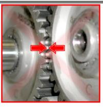
5- BEFORE APPLYING THE SEEGER, CHECK THE POSITION OF ALL GEARS AND THAT ALL REFERENCE MARKINGS ARE ALIGNED CORRECTLY.
